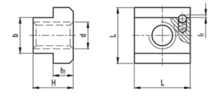
b -0.1 -0.3 = 18 d = M16 H = 20 h1 = 10 L = 28 I1 = 1.0 T-slot width DIN 650 = 18 Weight (g) = 68
